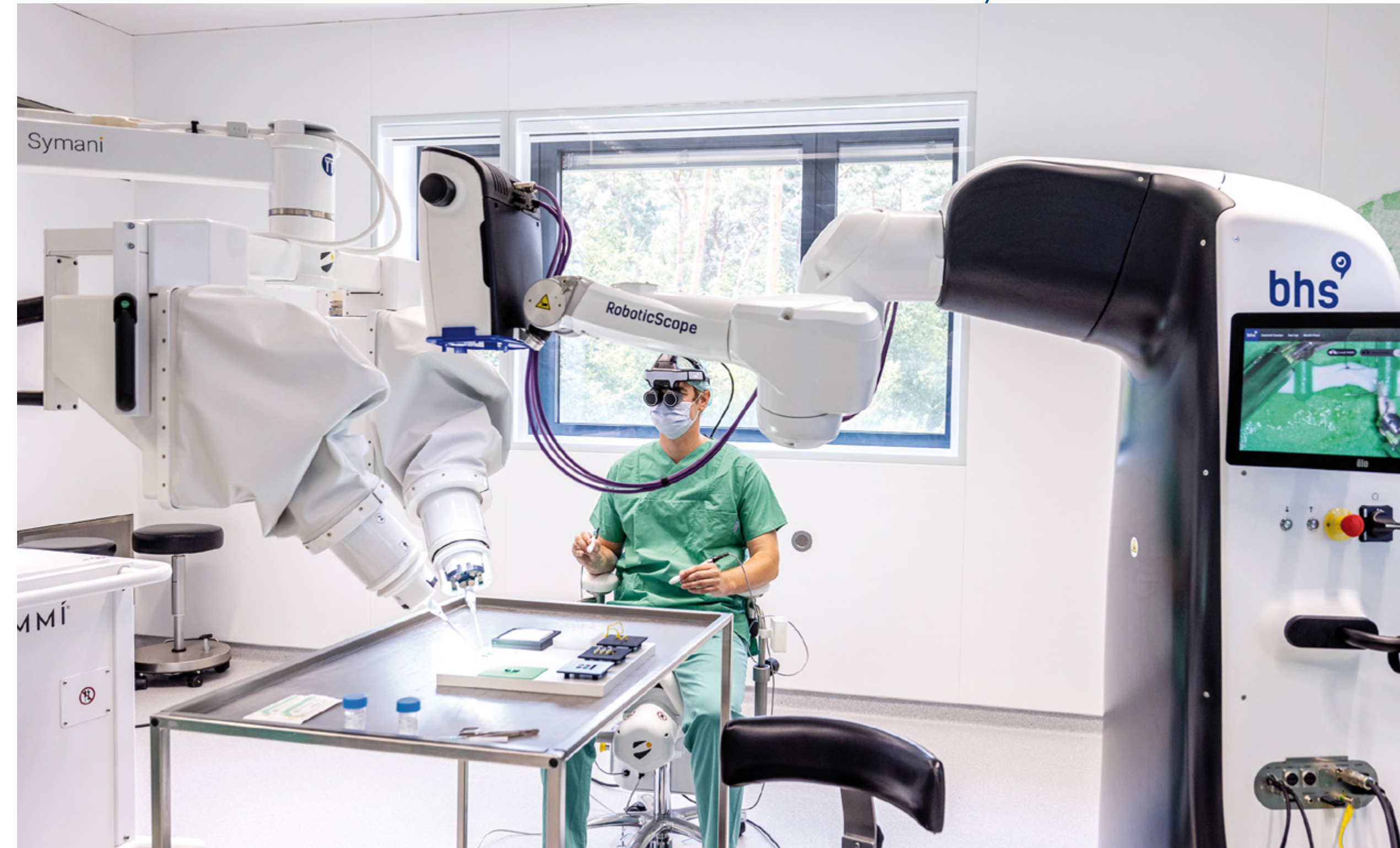
Dr Maximilian Kückelhaus with the surgical robot (left), which is linked up to a robotic microscope (right)
